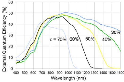
Fig. 5. External quantum efficiency of  $\text{Al}_x\text{In}_{1-x}\text{As}_y\text{Sb}_{1-y}/\text{GaSb}$  without GaSb top layer. All measurements were carried out with 200- $\mu\text{m}$  diameter APDs at 300 K.
