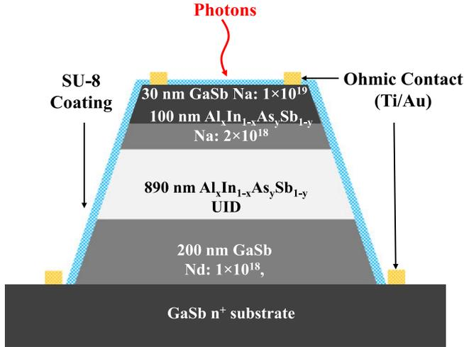
Fig. 2. Cross-sectional schematic of  $\text{Al}_x\text{In}_{1-x}\text{As}_y\text{Sb}_{1-y}/\text{GaSb}$  p-i-n APDs.
