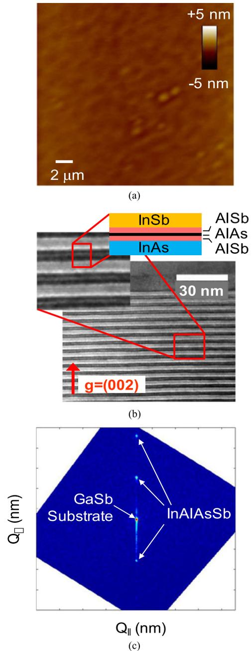
Fig. 1. Representative structural characteristics of  $\text{AlInAsSb}$  digital alloys illustrating the smooth morphology and well-defined interfaces. (a) Large-area atomic force microscopy, (b) bright-field transmission electron microscopy, and (c) (224) reciprocal space map for a 300 nm-thick  $\text{Al}_{0.5}\text{In}_{0.5}\text{As}_{0.5}\text{Sb}_{0.5}$  film. RMS roughness was  $\sim 0.25$  nm.
