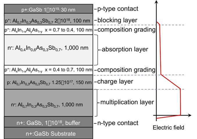
Fig. 7. Schematic cross section and electric field profile of  $\text{Al}_x\text{In}_{1-x}\text{As}_y\text{Sb}_{1-y}$  SACM APD.
