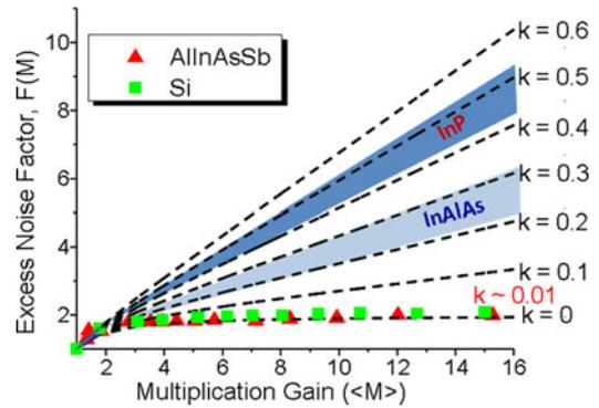
Fig. 10. Measured excess noise factor versus gain a 50- $\mu\text{m}$ -diameter  $\text{Al}_x\text{In}_{1-x}\text{As}_y\text{Sb}_{1-y}$  SACM APD (▲) and a commercial Si APD (■). The dashed lines are plots of the excess noise factor using the local field model for  $k$  values.
