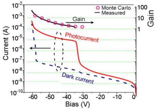
Fig. 8. Dark current, photocurrent, and measured and simulated (○) gain versus reverse bias of a 50- $\mu\text{m}$ -diameter  $\text{Al}_x\text{In}_{1-x}\text{As}_y\text{Sb}_{1-y}$  SACM APD at 300 K.
