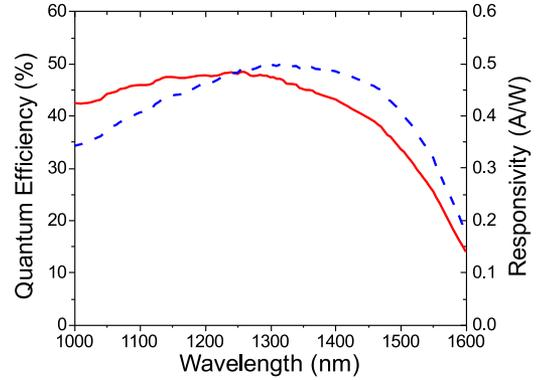
Fig. 9. External quantum efficiency and responsivity versus wavelength of a 150- $\mu\text{m}$ -diameter  $\text{Al}_x\text{In}_{1-x}\text{As}_y\text{Sb}_{1-y}$  SACM APD at 300 K.
