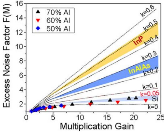
Fig. 6. Excess noise factor versus multiplication gain. The  $\blacktriangle$ ,  $\blacktriangledown$ , and  $\blacklozenge$  symbols represent the excess noise factor of  $x = 0.7, 0.6$  and  $0.5$   $\text{Al}_x\text{In}_{1-x}\text{As}_y\text{Sb}_{1-y}/\text{GaSb}$  APDs, respectively. Typical excess noise of InP, InAlAs and Si are shown by shaded region.
