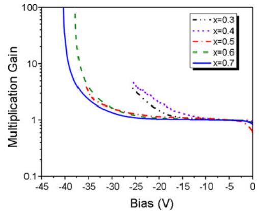
Fig. 4. Avalanche multiplication and measured photocurrents of  $\text{Al}_x\text{In}_{1-x}\text{As}_y\text{Sb}_{1-y}/\text{GaSb}$  APDs.
