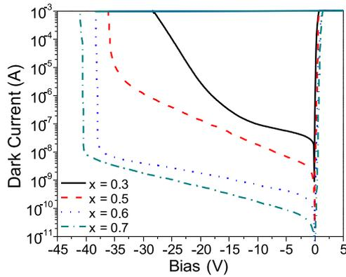
Fig. 3. Dark currents versus bias voltage of 50- $\mu\text{m}$ -diameter  $\text{Al}_x\text{In}_{1-x}\text{As}_y\text{Sb}_{1-y}/\text{GaSb}$  APDs.
