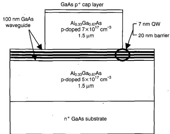
Fig. 1 Schematic diagram of GaInNAsSb ridge waveguide laser
