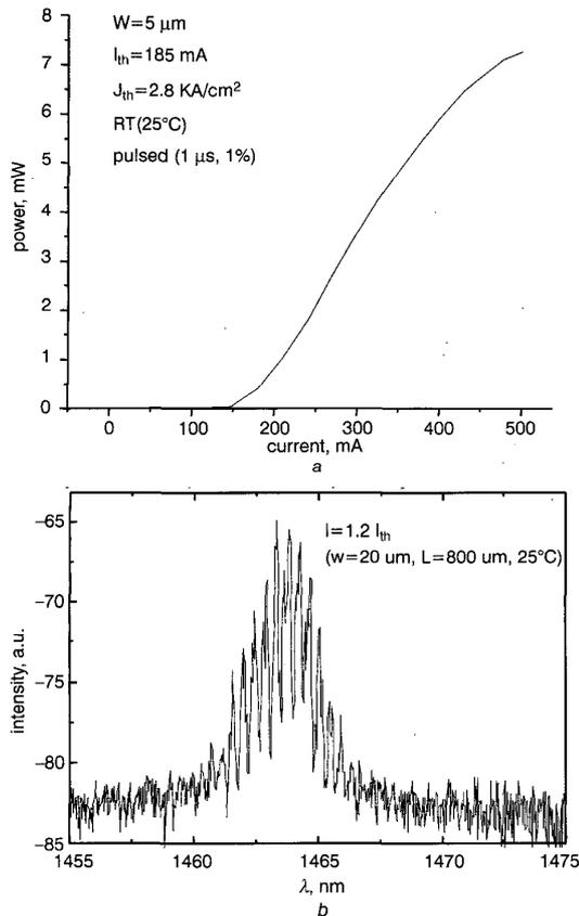
Fig. 3 L-I curve and optical spectrum for GaInNAsSb/GaNAsSb ridge waveguide laser with peak emission at 1.465 µm
