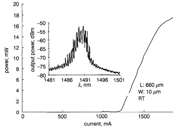
Fig. 4 L-I curve and optical spectrum for GaInNAsSb/GaNAsSb ridge waveguide laser with peak emission at 1.49 µm
