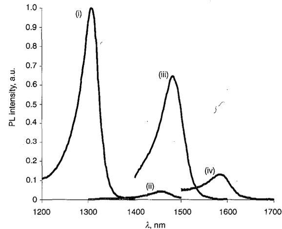
Fig. 2 Photoluminescence of various normalised GaInNAsSb samples
