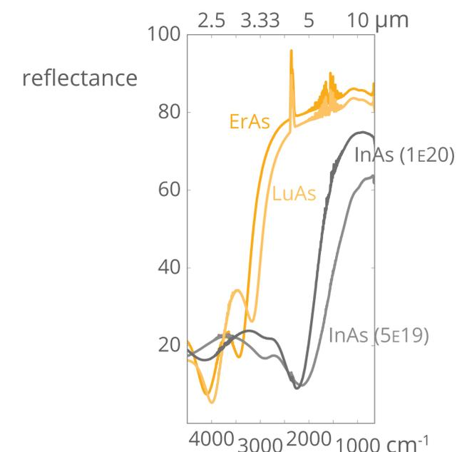
In addition to doped InAs, rare-earth / arsenic alloys also exhibit plasma frequencies in the mid-infrared. These semi-metals are also compatible with the GaAs materials system
