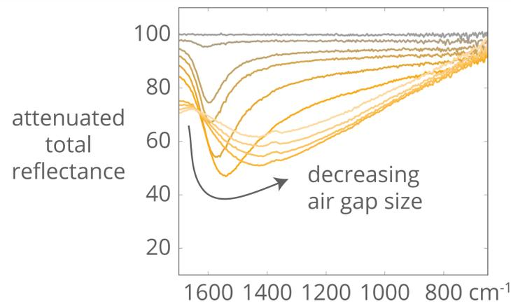
As we move the sample closer to the prism, we increase the local refractive index resulting in a red-shift of the peak. We find that an optimal air-gap size maximally couples light to the spp.
