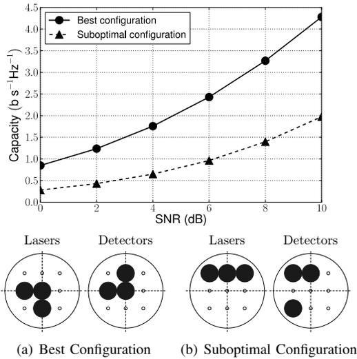
Fig. 6. Capacity vs. SNR for a  $3 \times 3$  MIMO system for the best device configuration and a suboptimal configuration in the plot above. The description of the subfigures is similar to that in Figure 5.
