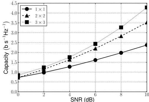
Fig. 4. Capacity vs. SNR for  $1 \times 1$ ,  $2 \times 2$ , and  $3 \times 3$  MIMO systems for the best device configuration
