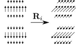
Fig. 2.  $\mathbf{R}^i$  describes rotation of the polarization of the electric field at section junctions
