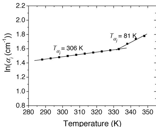
Fig. 10. Measured  $\ln(\alpha_i)$  for 20  $\mu\text{m}$  stripes as a function of device temperature (squares) extracted under pulsed (1  $\mu\text{s}$ , 1% duty cycle) operation to minimize device heating. Fits to experimental data are also shown (line). The increase in loss with temperature is a strong indication of IVBA.
