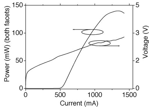
Fig. 6. CW  $L - I - V$  of a  $20 \mu\text{m} \times 2450 \mu\text{m}$  device.
