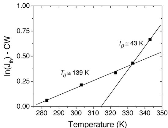
Fig. 8. Plot of CW  $\ln(J_{\text{th}})$  with temperature (squares) and the fits to an Arrhenius relation (lines) for a  $20 \mu\text{m} \times 2450 \mu\text{m}$  device. The  $T_0$  value for each temperature range is indicated.
