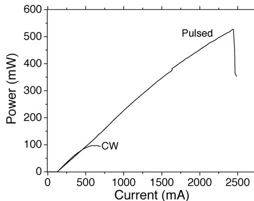
Fig. 12.  $L - I$  curves under pulsed and CW operation for an HR coated 10  $\mu\text{m} \times 983 \mu\text{m}$  laser. Peak output power was limited by COD under pulsed excitation and thermal rollover under CW operation.
