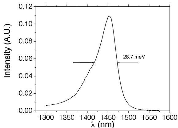
Fig. 1. Room-temperature PL spectrum of a single GaInNAsSb QW, with a linewidth of 28.7 meV.
