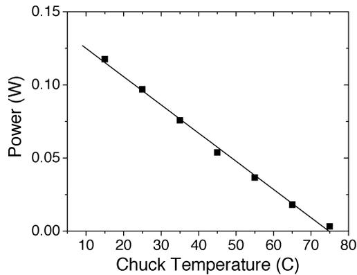
Fig. 13. Peak CW output power for an HR coated  $10 \mu\text{m} \times 983 \mu\text{m}$  laser as a function of ambient temperature (squares) and a linear fit (line). The increase in threshold and decrease in gain with temperature, along with slight increases in thermal and electrical resistance, produce a nearly linear relationship between peak CW output power and chuck temperature.
