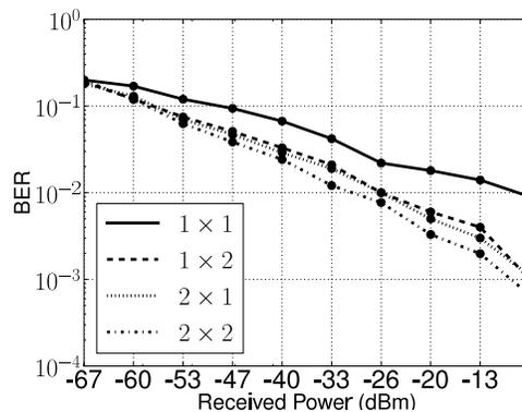
Figure 2. Measured BER vs. SNR for MIMO configurations
