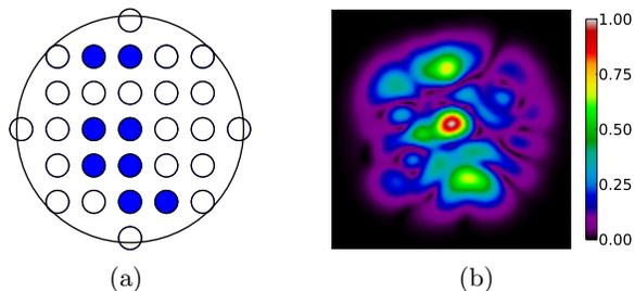
Figure 6. (a) The optimal subset of detectors (shaded blue) obtained by the algorithm for (b) a particular output modal pattern.
