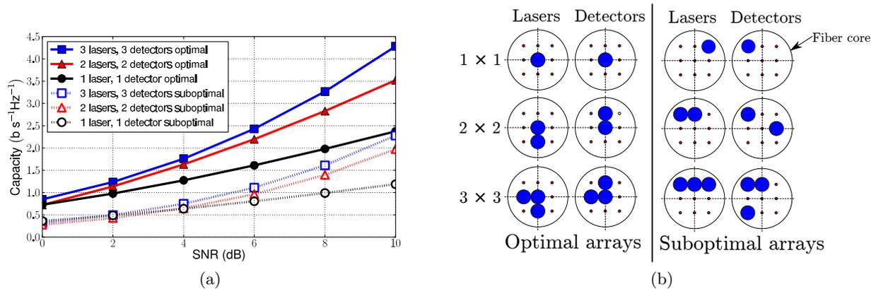
Figure 3. (a) Calculated capacity vs. SNR for  $1 \times 1$ ,  $2 \times 2$ , and  $3 \times 3$  MIMO systems for the best device configurations. (b) The optimal device configurations in each case. Note that severe penalties (40-50%) are incurred with the use suboptimal configurations.
