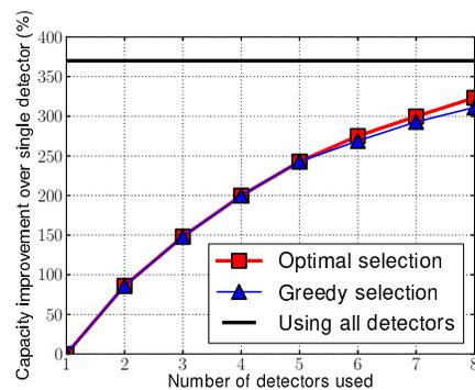
Figure 7. Capacity improvement with selected detectors: optimal (exhaustive) selection vs. greedy selection
