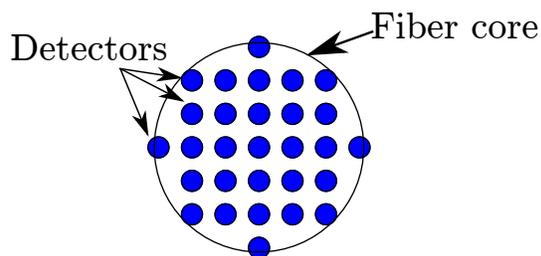
Figure 4. Detector array pattern used for the simulations, overlaid upon a 50  $\mu\text{m}$  fiber core. Photodetectors are 5  $\mu\text{m}$  in diameter, separated by a pitch of 8  $\mu\text{m}$ .
