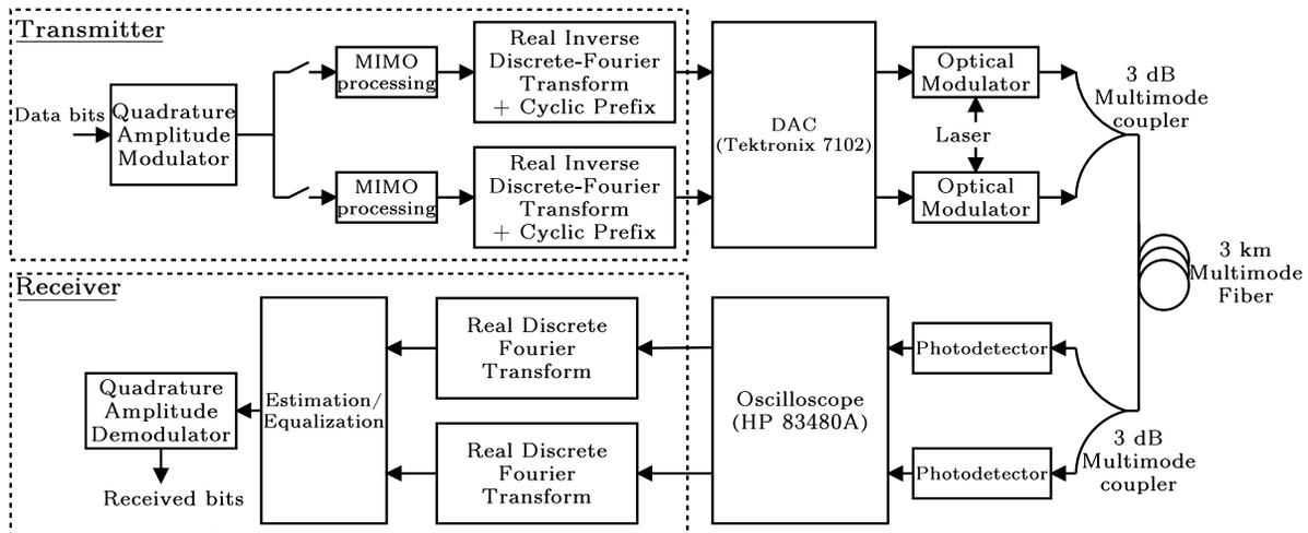
Figure 1. Schematic of the  $2 \times 2$  MIMO experimental setup: Used for  $1 \times 2$ ,  $2 \times 1$  and  $2 \times 2$  V-BLAST signaling
