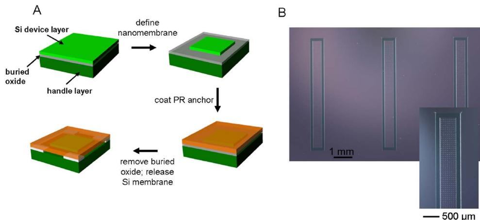
FIG. 4. (Color online) (a) Process flow for silicon nanomembrane fabrication from a SOI source wafer. (b) Nanomembranes after dry etching, but prior to photoresist anchor and HF undercut etching.
