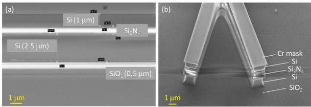
FIG. 10. (Color online) (a) Cross sectional SEM of a double bonded SOI wafer. The top dielectric is a  $\text{Si}_3\text{N}_4$  layer, while the second is  $\text{SiO}_2$ . (b) Cross sectional SEM of a splitter realized using double bonded SOI wafers.
