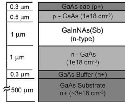
FIG. 1. Schematic of MBE-grown GaInNAs(Sb) devices.
