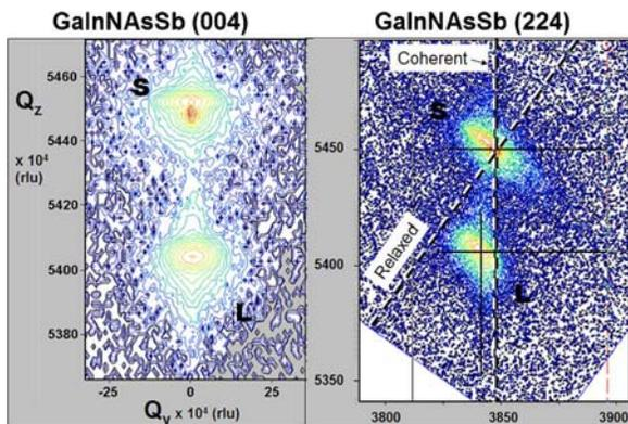
FIG. 10. (Color online) GaInNAsSb (004) reflection (left) and (224) reflection (right) reciprocal space maps ( $S$ =GaAs substrate reflection, and  $L$ =GaInNAsSb layer reflection). The center of each peak in the (224) (right) image marks the center of the reflection. The layer peak of the (224) reflection shows that the GaInNAsSb film is not completely coherent to the substrate, and has moved toward the line of relaxation.
