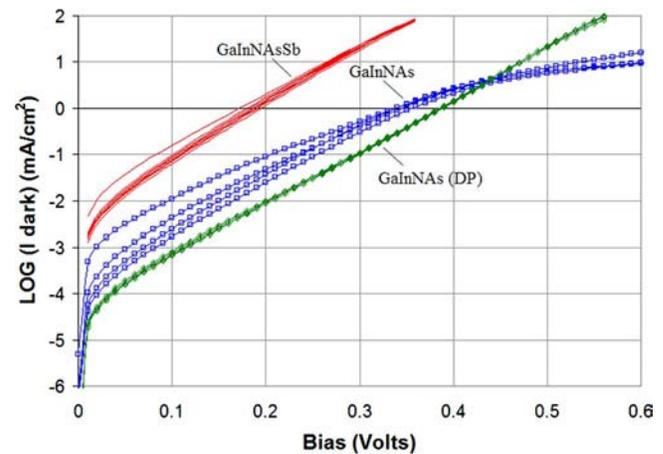
FIG. 5. (Color online) Semilog forward bias dark current-voltage characteristics of dilute nitride solar cells.
