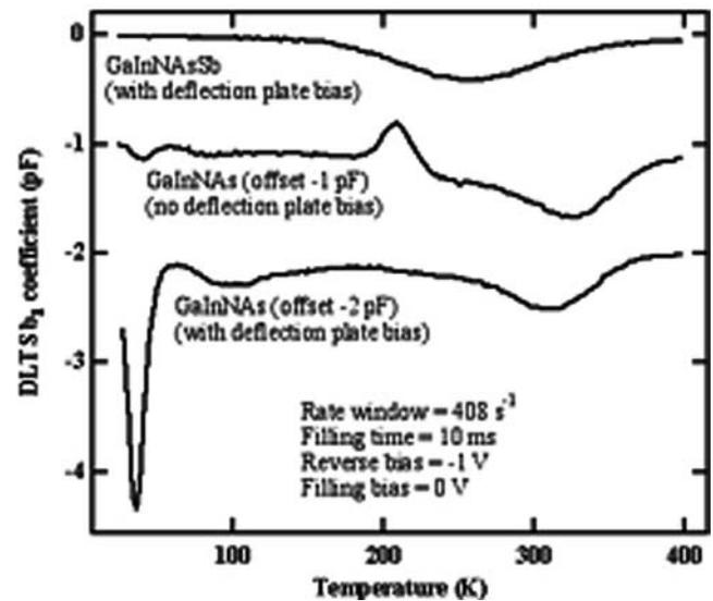
FIG. 7. Deep-level transient spectroscopy data.  $b_1$  Fourier coefficient of capacitance transients for all three samples. The downward-facing peaks represent electron traps and the upward-facing peaks represent hole traps.
