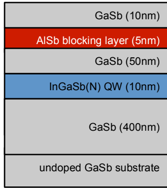
Fig. 1: Sample structure used for photoluminescence study. The AISb carrier blocking layer prevents recombination of photogenerated carriers at the surface.
